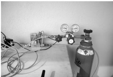
Fig. 6 Dosing equipment with massflow controller and tracer gas bottle (right)
