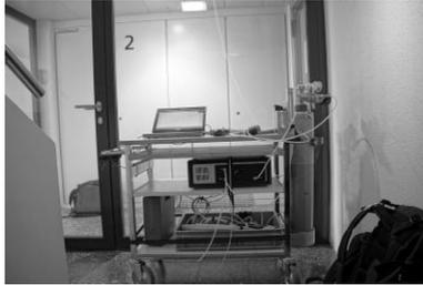
Fig. 9 Infrared-spectroscopy concentration measurement in the pressurized escape stairwell
